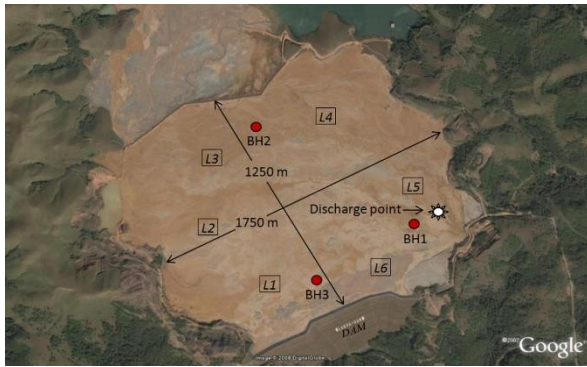
Figure 1. Top view of Lakya dam showing storage of iron ore tailings with sampling locations
