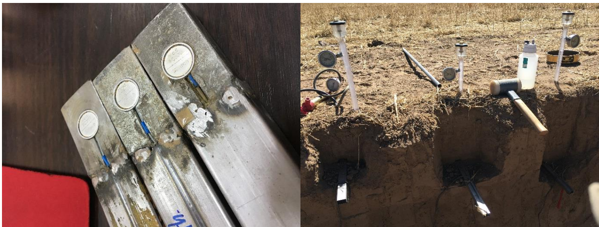
Figure 3. Load cells housings (left). Red Fill tensiometers installation and load cells lateral insertion at the predetermined depths of 15 cm, 30 cm and 45 cm.
