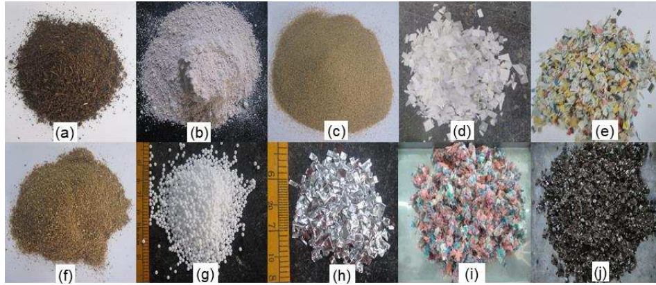
Figure 1: Components of SMSW: (a) Coco-pith (b) Kaolin clay (c) Fine sand (d) Polythene sheets (e) Newspaper (f) Saw dust (g) Thermocol beads (h) Aluminium foil bits (i) Cloth (j) Synthetic MSW
