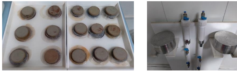
Figure 6. Filter paper (left). Haines' funnel (right)
