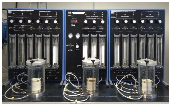
Figure 5. Flexible wall permeameter
