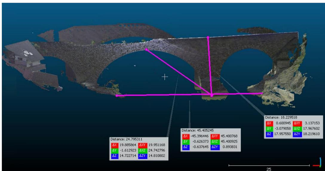
**Figure 15.** 3D point cloud excerpt derived from terrestrial LiDAR at the Altenahr double bridge. From left to right, measurements of the bridge clearance height ( $\Delta Z = 14.72\text{m}$ ), river cross sectional distance ( $\Delta X = 45.50\text{m}$ ), and total bridge height ( $\Delta Z = 17.96\text{m}$ ) were measured using the LiDAR derived point cloud.
