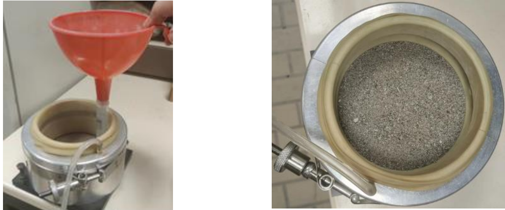
Figure 4. Dry air pluviation specimen preparation (left). Reconstituted specimen (right)
