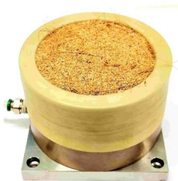
Figure 4. Closeup view of the prepared fiber reinforced test specimen
