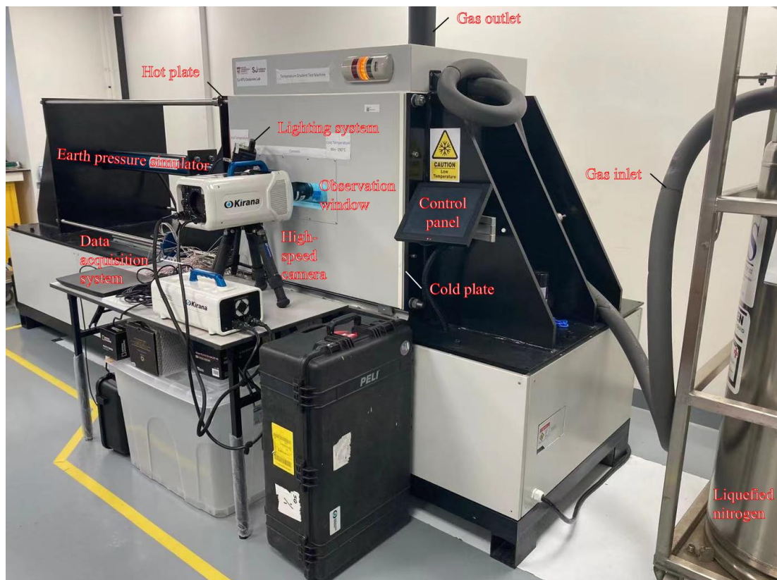
Figure 1. Laboratory setup of temperature gradient test system.
