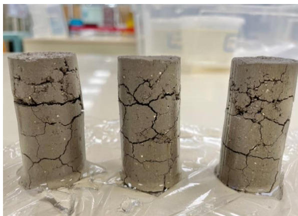
Figure 3. Compacted specimens with IBA/MC ratio of 5/5 soaked in seawater
