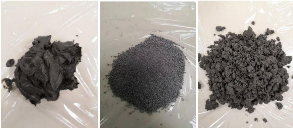
(a) (b) (c) Figure 1. Images of (a) MC, (b) fine IBA, and (c) IBA-MC with IBA/MC ratio of 5/5
