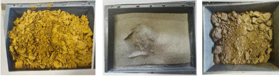
Figure 1. a) Loam Lembeek (loam), b) Artificial Soil (sand), c) Schist Clay (sandy loam)
