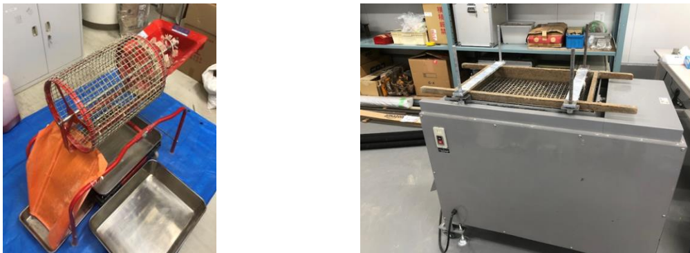
Figure 5. Rotary screen (left) and vibrating screen (right) used in the laboratory tests
