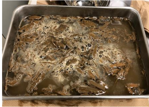
Figure 7. Gravimetric separation of soil and wood chips
