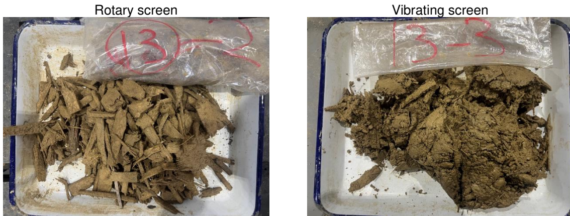
Figure 9. Appearance of residual materials generated from pilot-scale tests ( F_c15\% , w23\% )
