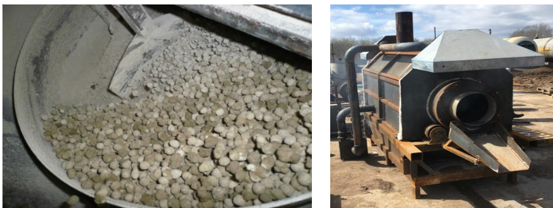
Figure 2. Production of a technogenic soil: left - production of raw pellets from sulphur-alkali waste and trepel in a pan pelletizer, right – the drum kiln.
