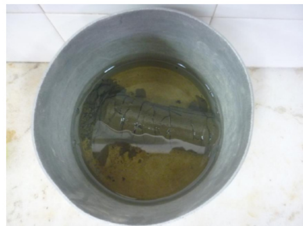
Figure 3. Cracking effect on a sample from the Gatun formation, which results from saturation.
