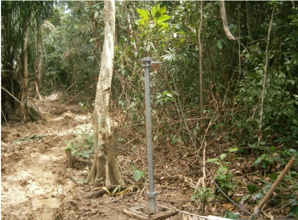
Figure 4. Gas gun used in this work.
