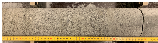
Figure 4. Frozen core sample of gravelly sandy Øysand soils.
