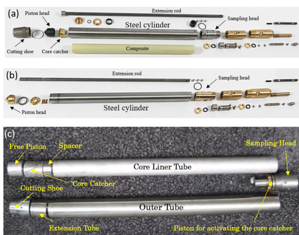
Figure 3. Piston samplers used: (a) Geonor-NGI PSØ54, (b) Geonor-NGI PSØ72 (www.geonor.no), and (c) Gel push sampler GPSØ71 (Kiso-Jiban, 2016).
