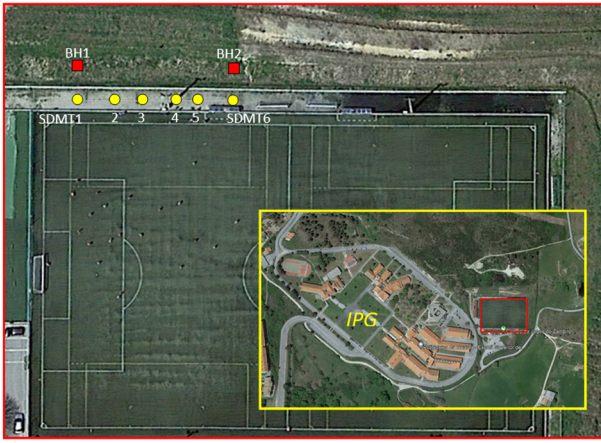
Figure 1. Position of the SDMT tests and boreholes (BH).
