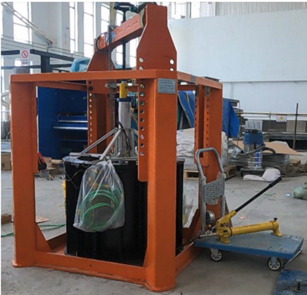
Figure 6. Pile installation frame.
