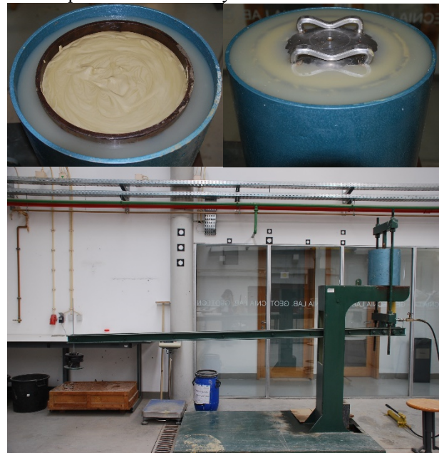
Figure 2. Slurry in the consolidation cell, prior to the placement of the drainage system and lid (top left); submerged cell, prior to load adjustment (top right); consolidometer (bottom).
