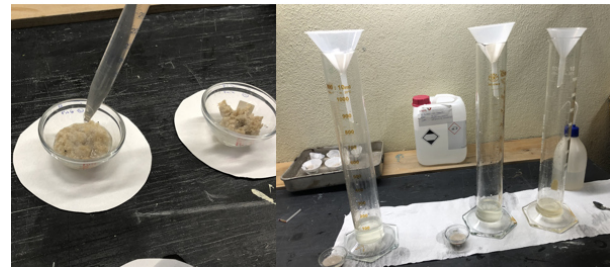
Figure 8. Leaching test to determine calcium carbonate content.
