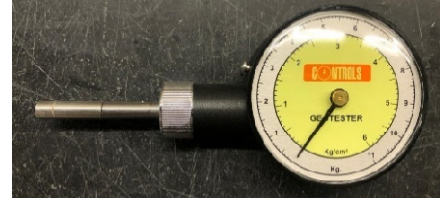
Figure 7. Penetrometer used for the tests (CONTROLS Geopocket).
