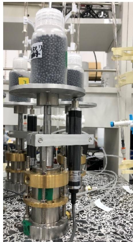
**Figure 2.** Swelling deformation apparatus with multi-ring mould.
