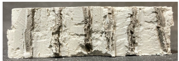
(c) at 80% of peak strength in residual stage, (2.03 mm of horizontal displacement)
