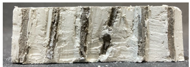
(a) at 80% of peak strength, (0.39mm of horizontal displacement)
