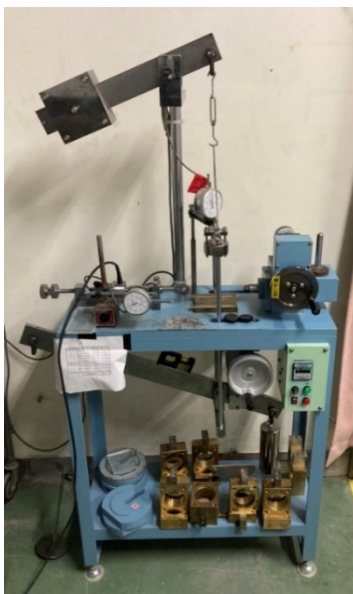
Figure 2. Direct shear apparatus and shear boxes on the lower table.
