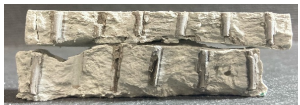
(d) at 50% of peak strength in residual stage, (9.14 mm of horizontal displacement)
