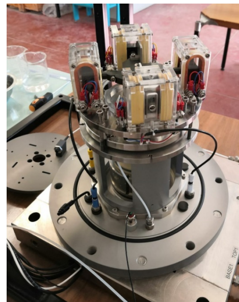
Figure 2. Resonant column / Torsional shear apparatus available at the Geotechnical Laboratory of the University of L'Aquila: compressed air cell (a) and pedestal, specimen, and driving system (b).
