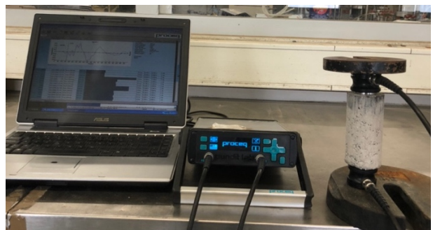
Figure 5. Equipment for carrying out the P-wave and S-wave test – PunditLab.
