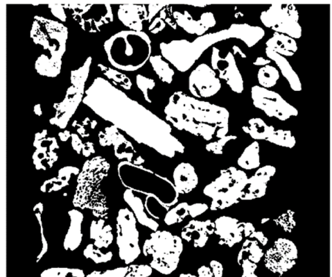
Figure 4. Sharpened and thresholded, using Otsu method, image of the São Tomé sand in a 30 mm diameter tube.
