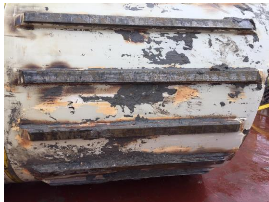
b. Clay traces between the ribs of the follower (exterior).
