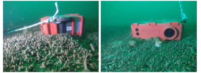
Figure 1 – 4-component seismic sensors (Sercel GPR nodes) placed on the seabed (28 m depth)
