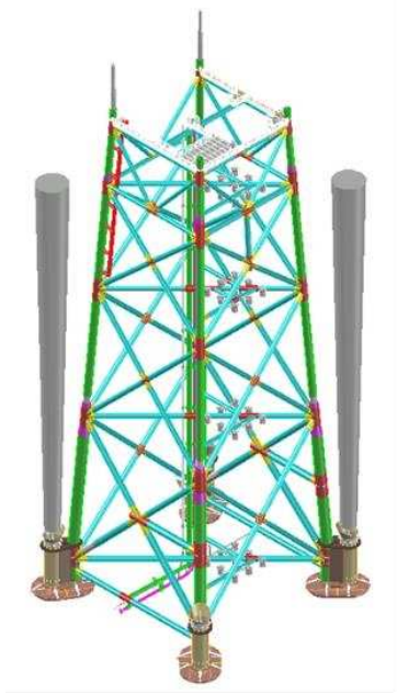
Figure 5. Clearance check for stabbed pile only with jacket structure for sea state of H_s=5.7\text{m} .
