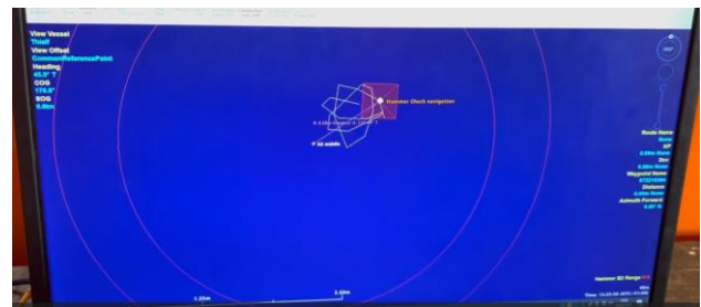
Figure 11. Traces of the hammer top movement during pile driving operation.
