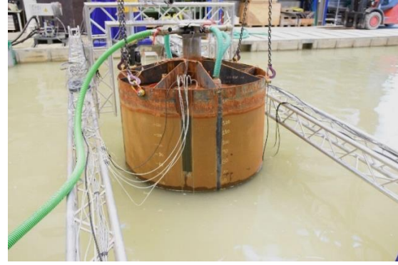
Figure 2 – Overview of experimental setup: Sensors applied and forces acting on a caisson during suction installation (left). Installation of the suction caisson with D = 1.60 m and L = 1.42 m in the geotechnical test pit of the TTH (right)
