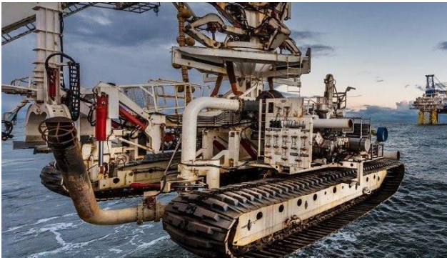
Figure 2. Typical subsea mechanical chain cutter
