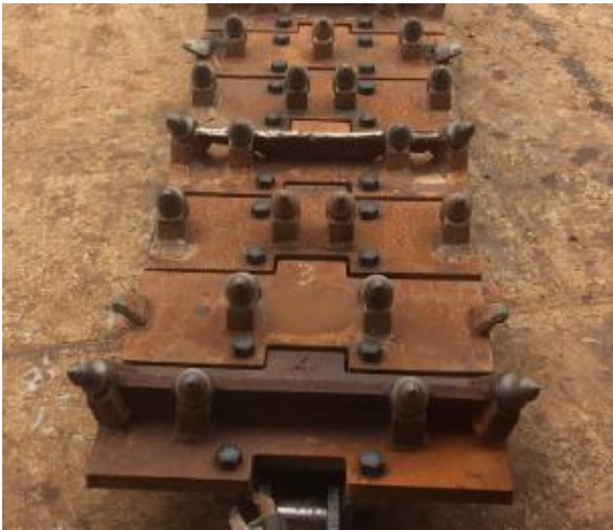
Figure 5. Cutting chain to show pick pattern
