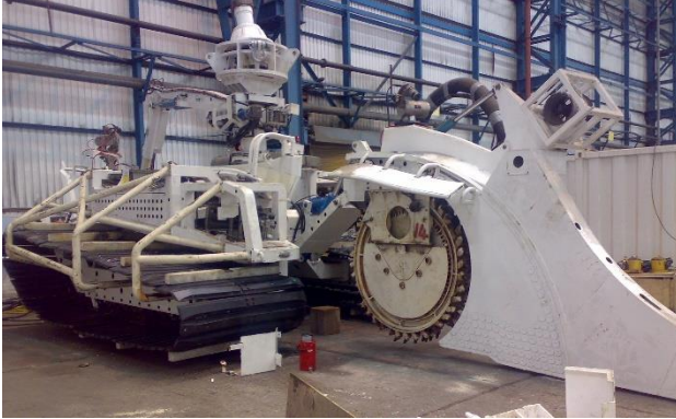
Figure 1. Typical subsea wheel cutter
