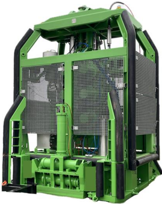
Figure 1. Infinity SCPT seafloor pushing apparatus (frame) and its side-mounted seismic hammer source.
