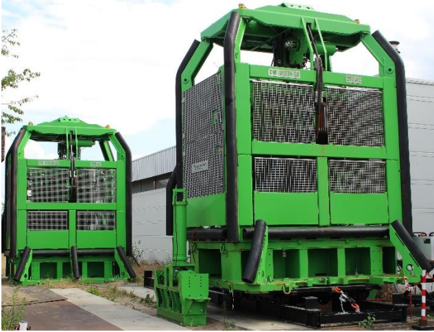
Figure 4: Seabed CPT system (ROSON-3D-ST) with seismic source
