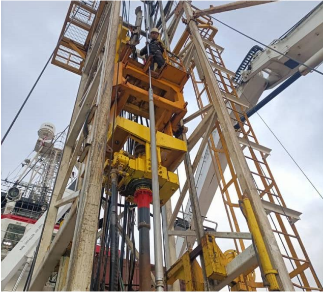
Figure 1: Wireline CPT system (WISON-APB)
