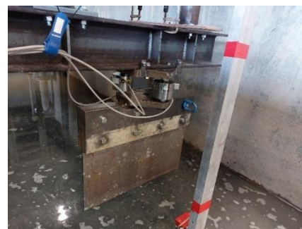
Figure 1. An impression of the testing assembly with an instrumented intruder (plate)
