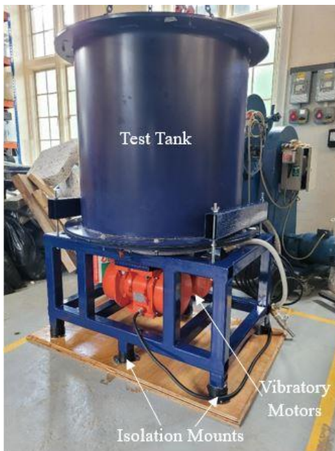
Figure 2 Vibratory table, used in saturated sand sample preparation.
