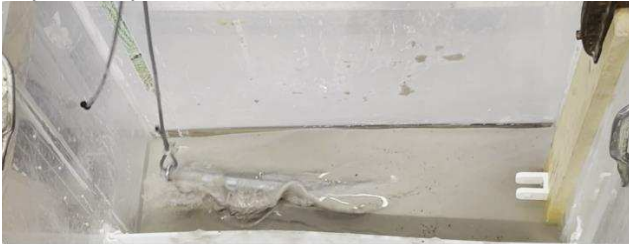
Figure 7: pullout of rigid cable (steel rod). Dilation observed along entire length of rod
