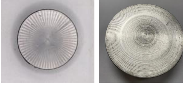
Figure 2 - Smooth (left) and rough (right) faces of the steel disk used as the shear interface for constant normal load and constant normal stiffness interface tests
