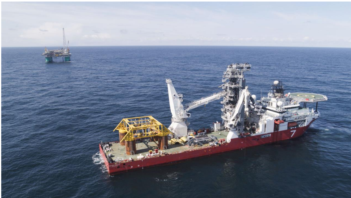
Figure 1 – Typical foundation structure for template
