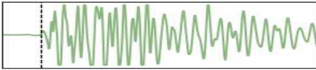
Figure 1 – P-wave shot (unfiltered); near and far traces show clear first arrival visibility and no/low noise (high confidence); overall shot confidence is high
