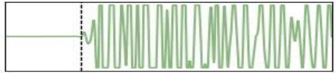
Figure 1 – P-wave shot (unfiltered); near and far traces show clear first arrival visibility and no/low noise (high confidence); overall shot confidence is high
