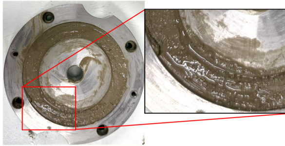
Figure 6. Example of shear tracks and striations from interface ring shear test (10 \mu\text{m} surface roughness and 5 kPa normal stress).
