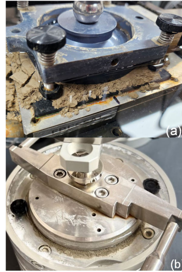
Figure 5. Soil loss from (a) interface shear box and (b) interface ring shear tests ( 0.02 \mu\text{m} surface roughness and 50 kPa normal stress).
