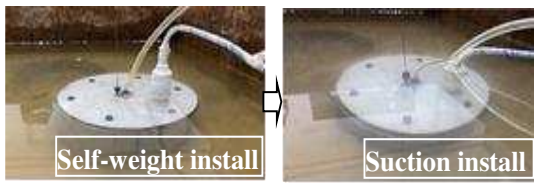
Figure 3. Suction installation test of bucket foundation
