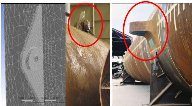
Figure 74 left) fabricated pad-eye for temporary moorings and right) typical cast pad-eye for permanent moorings.
