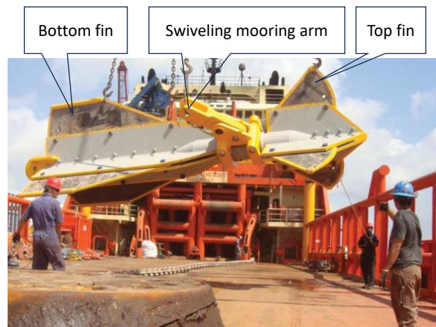
Figure 76 Typical OMNI-Max ® Mk2 anchor (picture from https://delmarsystems.com/products/anchors/omni-max/ ).
