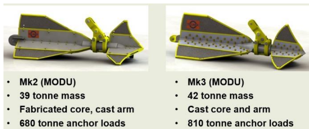
Figure 79 Comparison of OMNI-Max ® Mk2 and Mk3 anchors (from Delmar, 2024).
