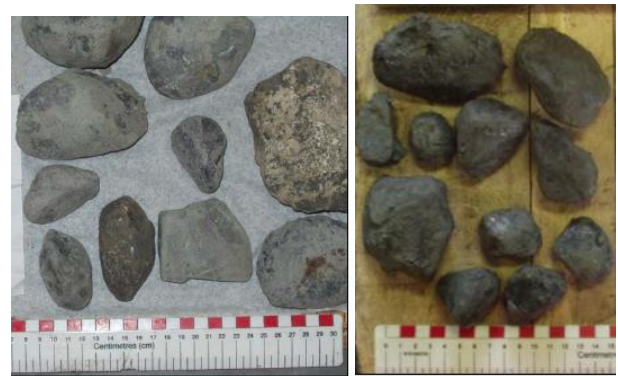
Figure 35 Cobbles recovered in the drill out activities inside Piles P7 (left) and P8 (right)
