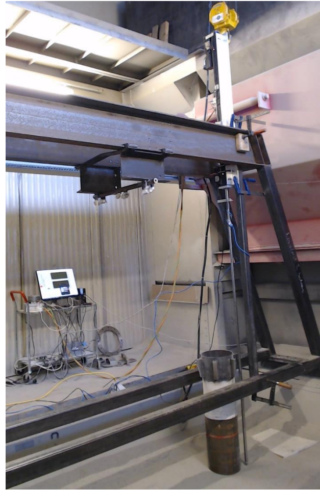
Figure 2. Test Setup for CPT after pile driving
