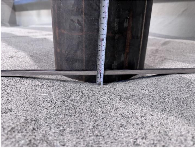
Figure 4. Settlement due to densification around the pile
