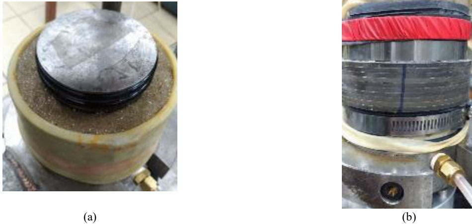
Figure 1. Photos of Torsional shear box: (a) specimen with outer membrane, (b) and assembly of shear box.
