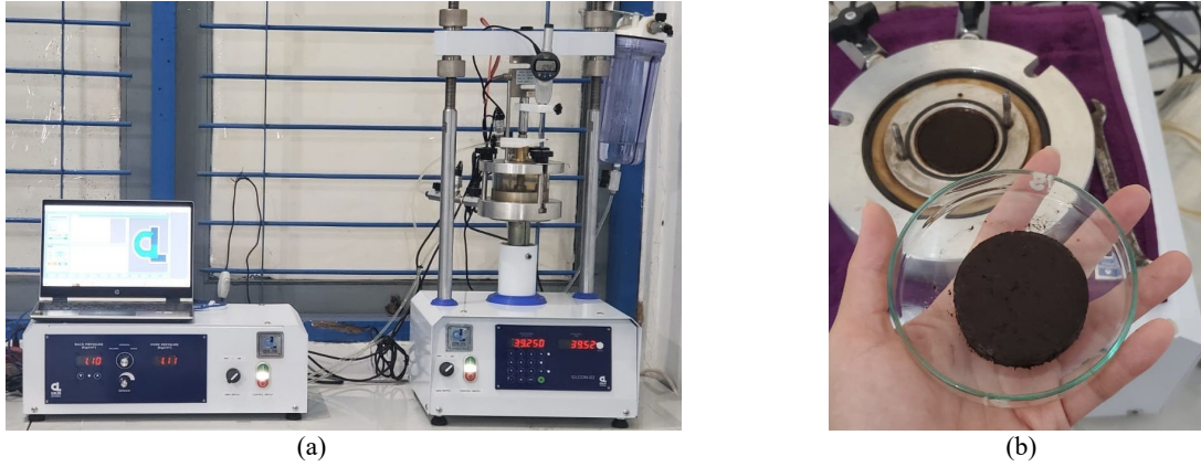
Figure 2. Constant Strain Rate (CRS) test: (a) apparatus and (b) specimen after test.
