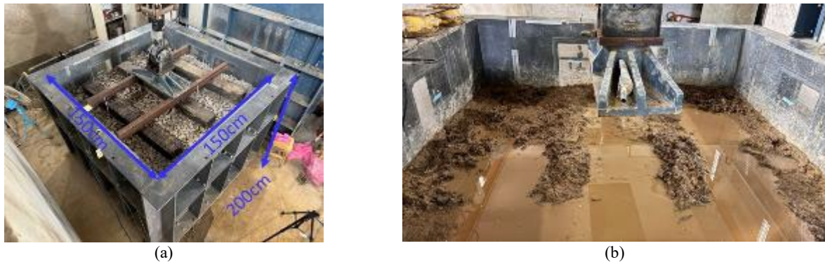
Figure 1. The before and after of the cyclic-loading test using the large-scale soil box: (a) the large-scale soil box used in this experiment and (b) the post-experiment results.
