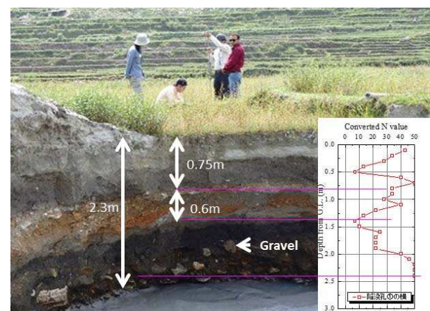
Fig. 5 Soil profile and DCPT result in the location 2 observed in Sinkhole on June 2014 (Kuwano, et al., 2014)
