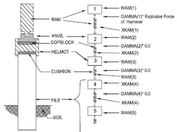
Fig.1 Pile Idealization for Wave Equation Analysis
