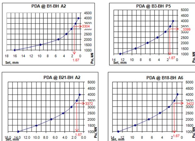
Fig. 2 Load capacity vs set graphs
