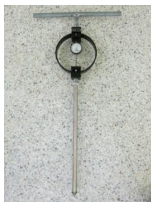
Fig. 2 Cone penetrometer for cone tip resistance measurement before and after explosion
