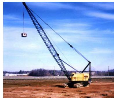
Fig. 1 A crane operated DDC unit
