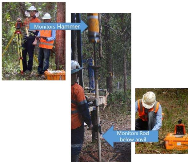
Fig. 2 PDM monitoring of SPT
