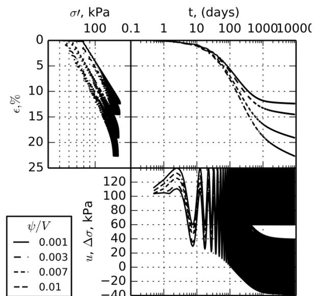
Fig. 4 Effect of  $\psi$  on consolidation, cyclic load
