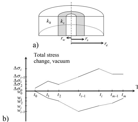
Fig. 1 a) Axisymmetric unit cell b) Piecewise linear surcharge and vacuum loading.
