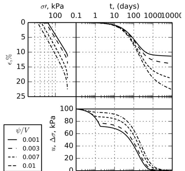
Fig. 3 Effect of  $\psi$  on consolidation, instant load
