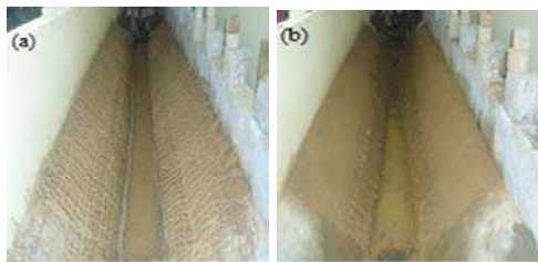
Fig. 4 River model with geotextile mat and cocolog (a) before experiment (b) after experiment
